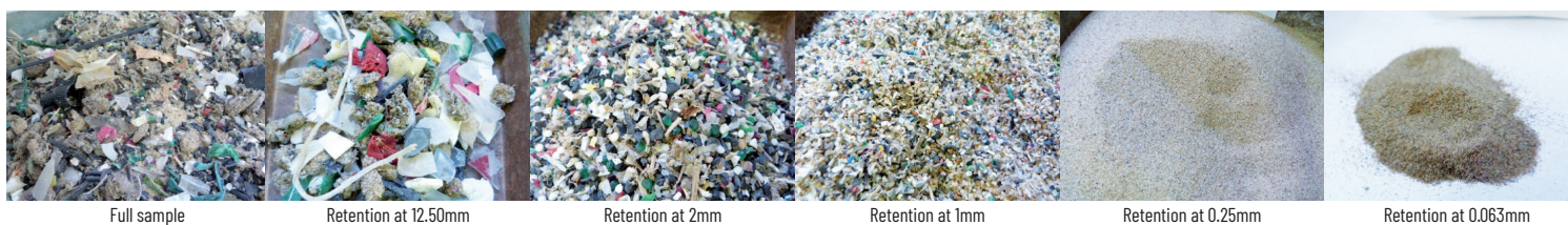
Particle-size test of a sample from a DA Defender® installed in a plastics factory.
