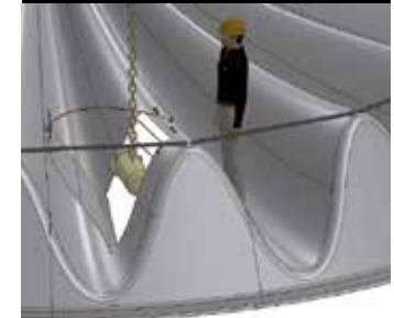
Access window in stirrers
