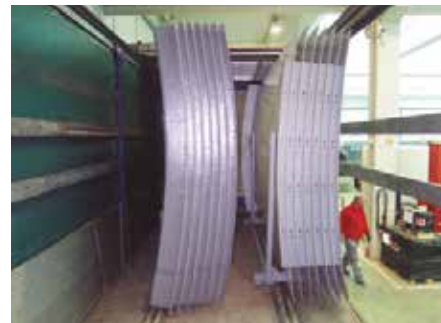
W-Tank® with H=11m, D=13.2m and 1,505m 3 capacity transported in a lorry.
